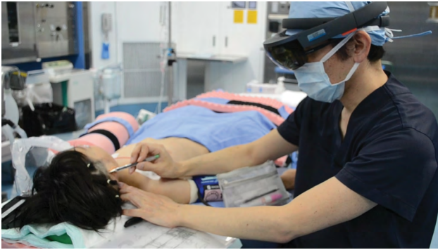
Fig. 1. The prepared 3D images were projected onto the surgical field using HoloLens. The surgeon can confirm the position of the auricle through the device.
