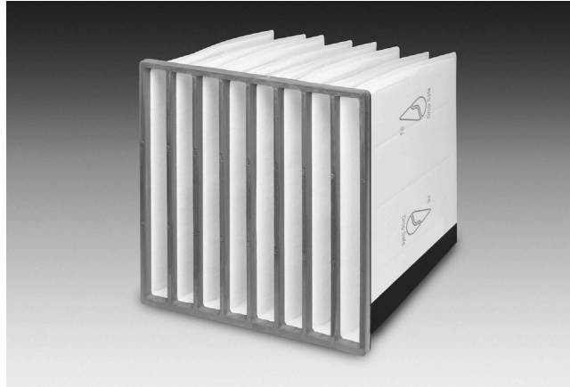
Figure 3.41 Pocket filter to remove airborne particulate matter as well as snow, mist and fog, acting as a combined filter and water coalescer. The Filtrair Drop Safe is designed for the elimination and drainage of free water and air borne salt crystals.
