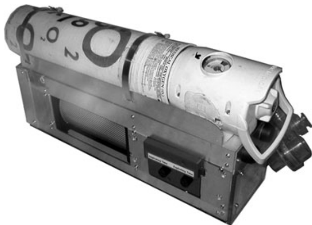
Figure 2 Design (i): original design for adverse environments/patient transport. With the integrated lightweight 460-l C/D cylinder shown, this would have an endurance of up to 7 h with no oxygen re-supply.
