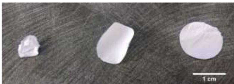
Figure 2. Image of electrospun fiber substrates ( 1.267 \text{ cm}^2 ). From left to right: SG 80A/HP 93A, TP 470/SG 80A, and TP 470/HP 93A.
