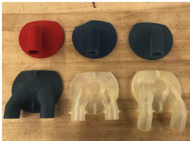
Fig. 2. 3D-printed manifold was designed to mate to where the fan cover can be removed from the Flyte helmet.
