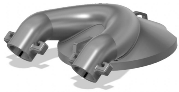
Fig. 7. Moved the ports outward to allow for the rectangular Pall BB50T filter on 4/2/2020.
