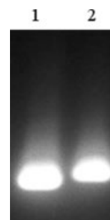
Figure 2. The conjugation pattern on 2.5% agarose gel electrophoresis was examined at UV excitation wavelength 345 nm, showing a different band pattern between free QDs (lane 1) and QDs-conjugated aptamer (lane 2).
