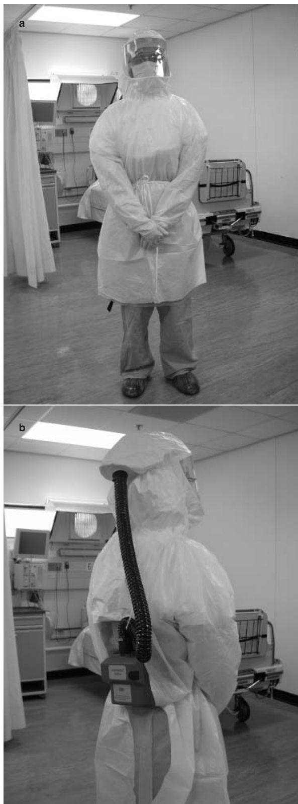
Figure 1 Powered air purifying respirator (PAPR) (Air-mate). (a) Frontal view. (b) Back view of battery with HEPA filter and duct supplying purified air to hood unit.
