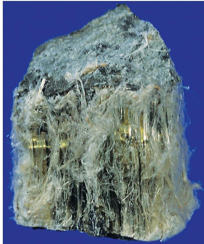
Figure 7.1.19 A sample of Quebec chrysotile showing the fibrous nature of the ore.
