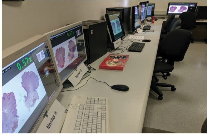
Fig. 1 The evaluation set-up. Each of the displays was set-up within a window-less room with fixed artificial lighting. The same WSI was shown on each display for side-by-side comparison.
