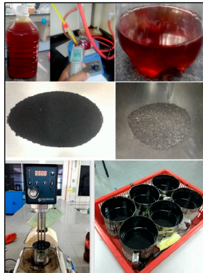
Figure 6. Asphalt binder (bottom right) modified with waste cooking oil (top), crumb rubber (middle left), palm oil fuel ash (middle right), and the blending process (bottom left) [22].
