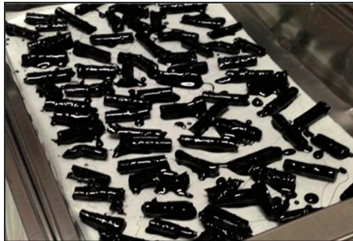
Figure 12. Encapsulated cigarette butts (CBs) used in the research conducted by Mohajerani et al. (2017) [71].
