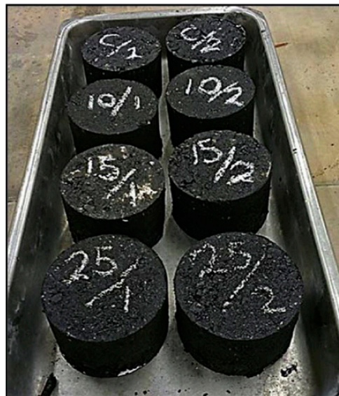
Figure 13. Some CB-modified asphalt samples prepared by Mohajerani et al. (2017) [71].
