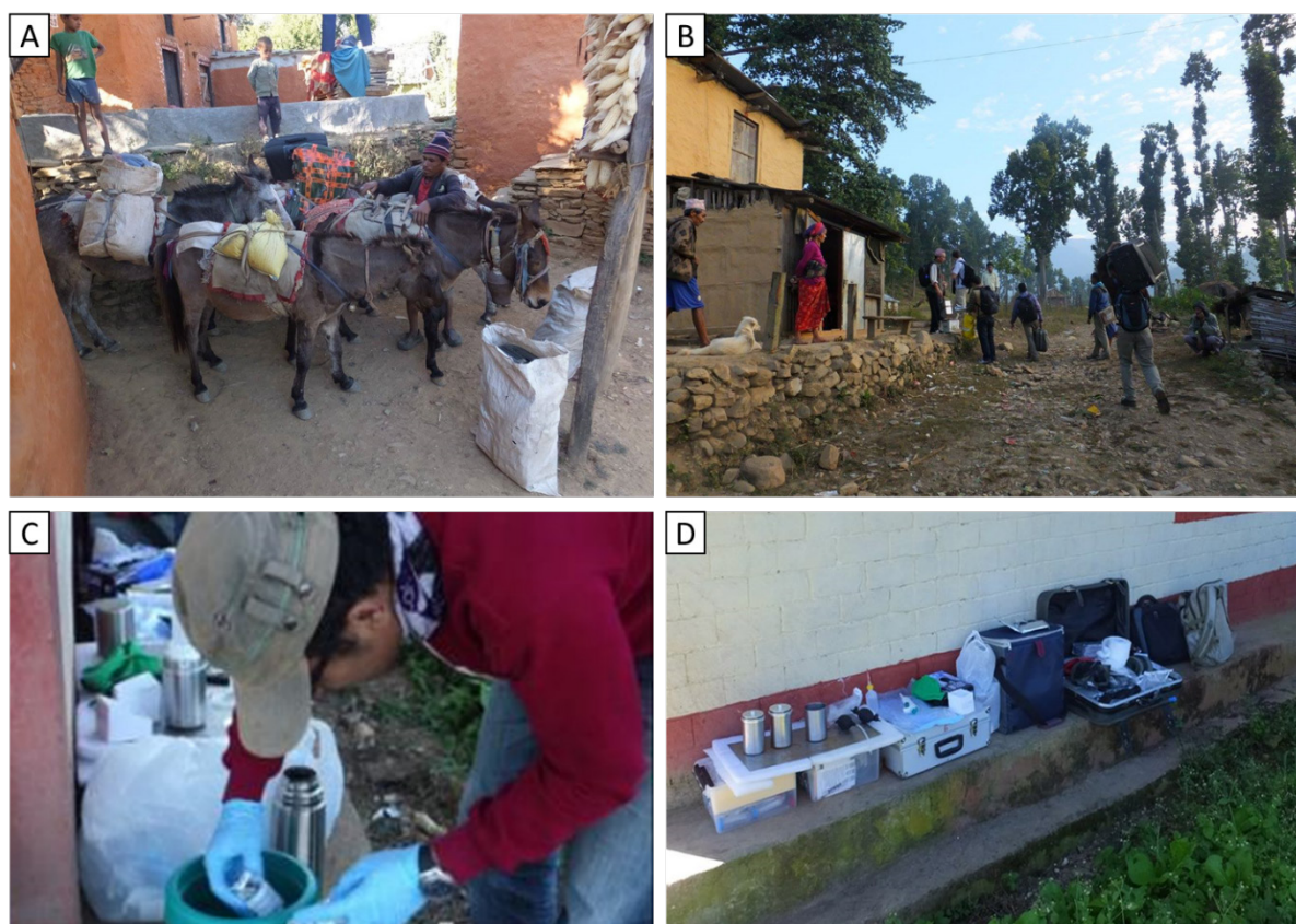
Figure 2. (A): Mules for transporting lab equipment. (B): Carrying equipment to a location without road access. (C): Thermos bottle to transport samples. (D): Adaptable field water testing kit including solar-powered incubation system.
