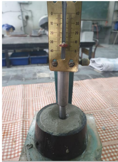
Figure 5. The view oement paste with MSWI slag under Chateliera's test (authors' photo).
