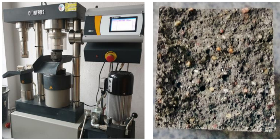
Figure 10. The view of compressive strength and tensile strength testing of mortars in the automatic apparatus and sample fracture structure (authors' photo).
