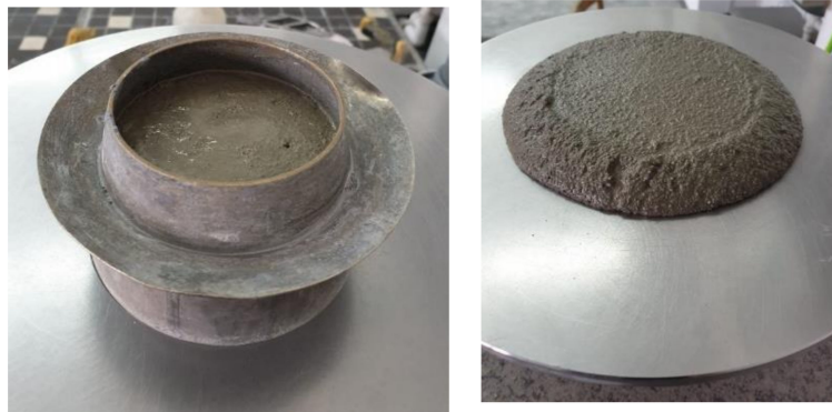
Figure 8. The flow of fresh mortar with the addition of 30% of MSWI slag after shaking 15 times (authors' photo).
