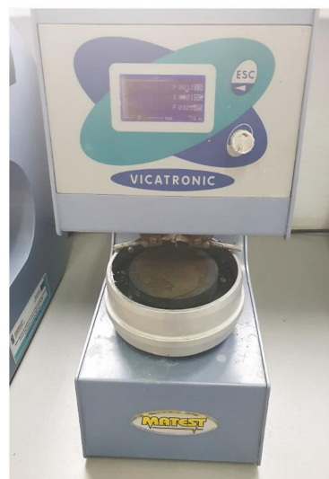
Figure 7. The view of cement paste with MSWI slag in automatic Vicastronic under measuring setting time (authors' photo). No volume change of cement paste was observed under measuring of setting time, which could affect the correct measurement.
