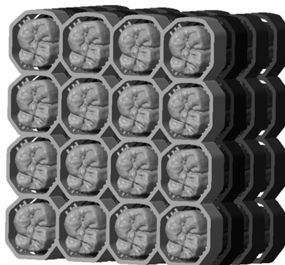
Figure 12. 'Milling' support enables stacking and stringing together.
