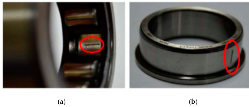
Figure 1. Bearing fault conditions. (a) bearing crack on the outer surface; (b) bearing crack on the inner surface.
