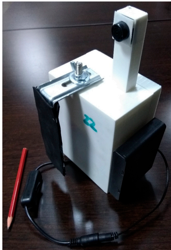
Figure 3. External casing for the chair–stand sensor. The sensor can be attached to chairs with very different designs thanks to a hook of adjustable width. The ultrasound sensor towers above like a periscope.
