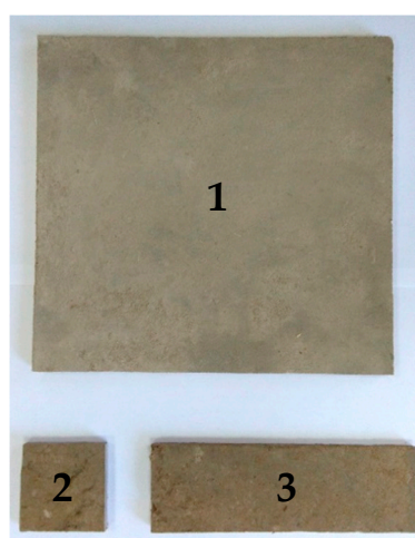
Figure 2. Specimens for the different tests. 1 ( 300 \times 300 \text{ mm}^2 ), 2 ( 50 \times 50 \text{ mm}^2 ), 3 ( 150 \times 50 \text{ mm}^2 ).
