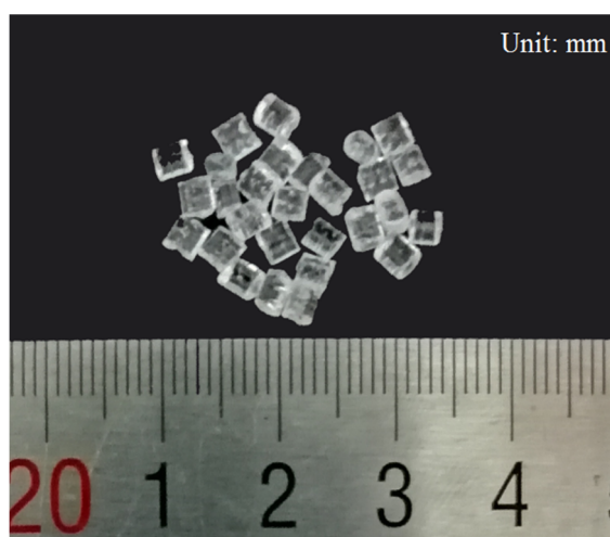
Figure 4. The amount of raw COC plasticized each time.
