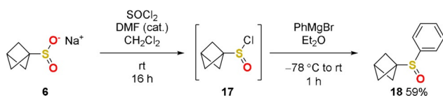
Scheme 4. Chlorination of 6 and subsequent reaction with phenylmagnesium bromide to sulfoxide 18 .
