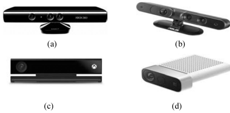
Figure 1. (a) Kinect v1; (b) Asus Xtion PRO LIVE; (c) Kinect v2; (d) Azure Kinect DK.
