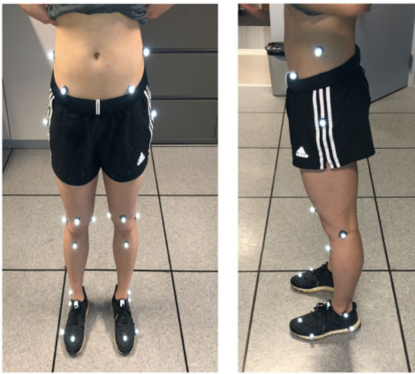
Fig. 2. Anterior and lateral views of the 28 passive retroreflective markers used for motion analysis.
