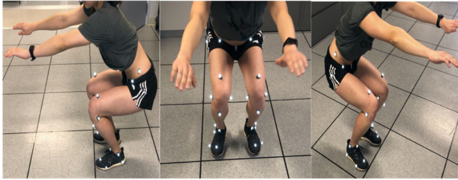
Fig. 1. An instrumented participant demonstrates an unrestricted squat where they were instructed to squat as low as possible while keeping their upper limbs parallel to the floor and feet shoulder width apart.
