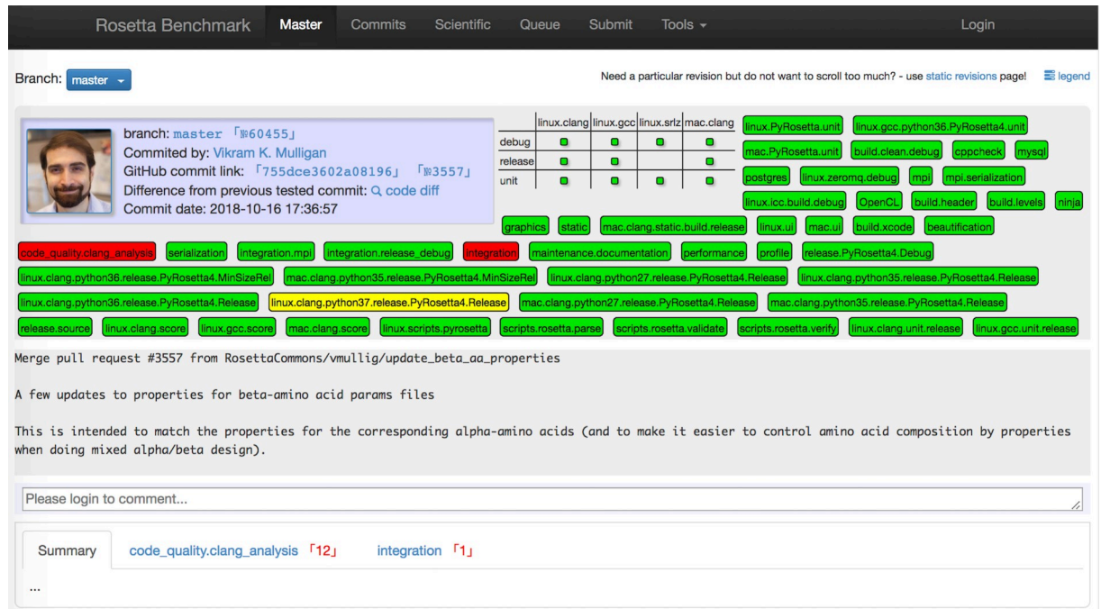
Fig 4. Software testing. Testing is essential to ensure stability and correctness of software. This is a view of our testing server dashboard for a specific merge into the master branch of Rosetta. We continuously run a large number of tests, such as build tests, unit tests, integration tests, performance tests, code analysis tests, and scientific benchmarks. Tags in green, red, and yellow denote test pass, failure, and currently running.
