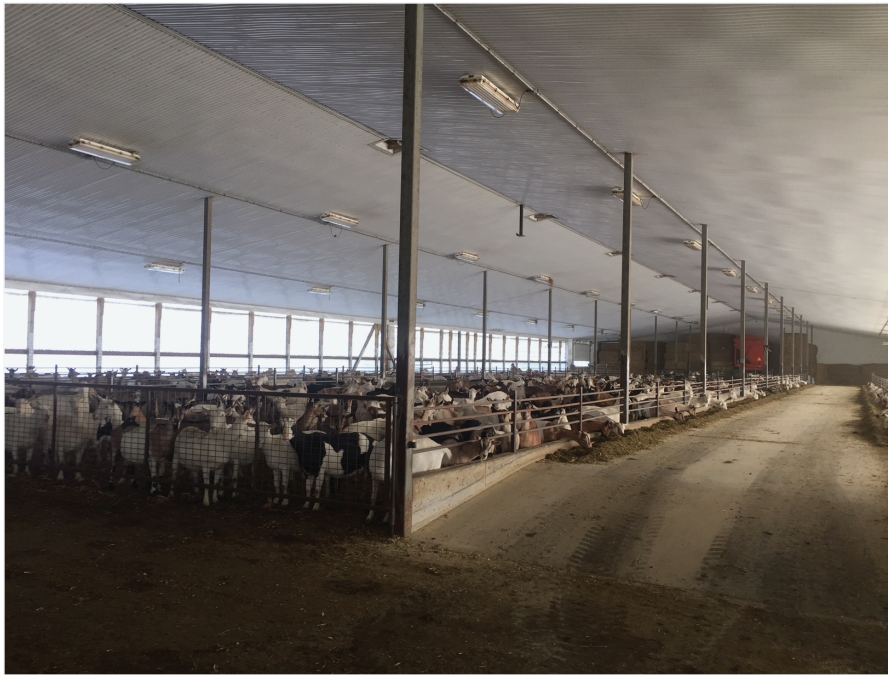
Figure 3. Commercial dairy goat farm (Henry and Anja van der Vlies and family, Ontario, Canada) promoting eye-level feeding posture by elevating the drive alley.
