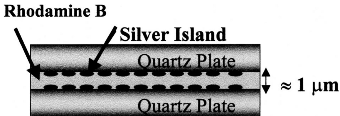
Fig. 2. Sample geometry. Two silver islanded quartz plates sandwich \approx 1 \text{ mm} RhB solution. Given that metal-fluorophore interactions are thought to extend some 200 \text{ \AA} into the solution, in this sample geometry only \approx 4\% of RhB molecules are within this active region. This suggests that the true enhancement effect in Fig. 1 is at least 25 times higher.
