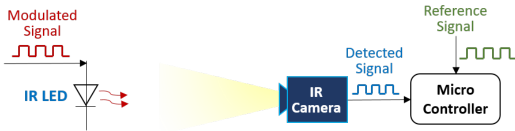
Figure 5. Schematic of the signal modulation for the transmitter (IR LED) and the receiver (IR camera with a Microcontroller).
