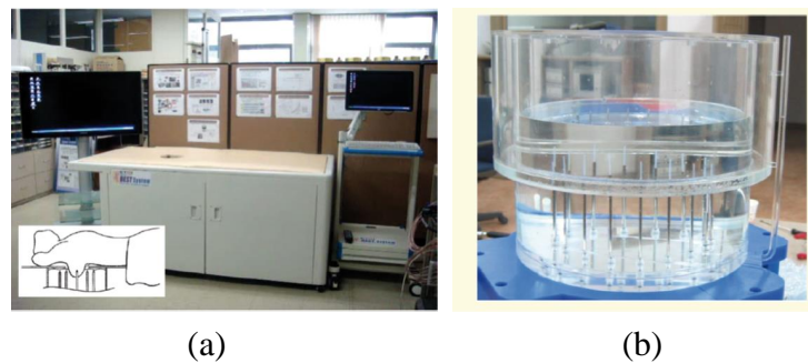
Figure 7. A prototype imaging system developed by Son et al. [68]. (a) View of the entire system. (b) View of the breast holder showing the antenna array in the liquid bath. Reprinted with permission from [68].
