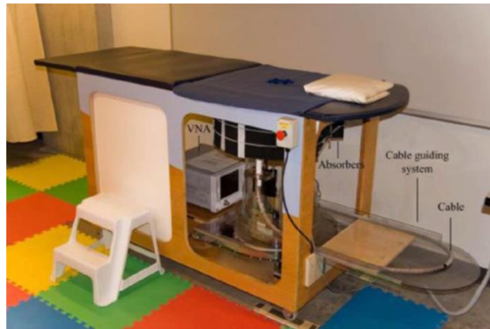
Figure 18. Tissue sensing adaptive radar (TSAR) prototype radar-based MI system for breast cancer detection developed by Fear et al. [78]. Reprinted with permission from [78].
