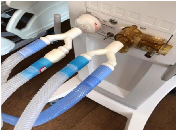
Fig. 2 Image showing a 3D printed ventilator splitter designed by an orthopedic surgeon with his 3D printing team
