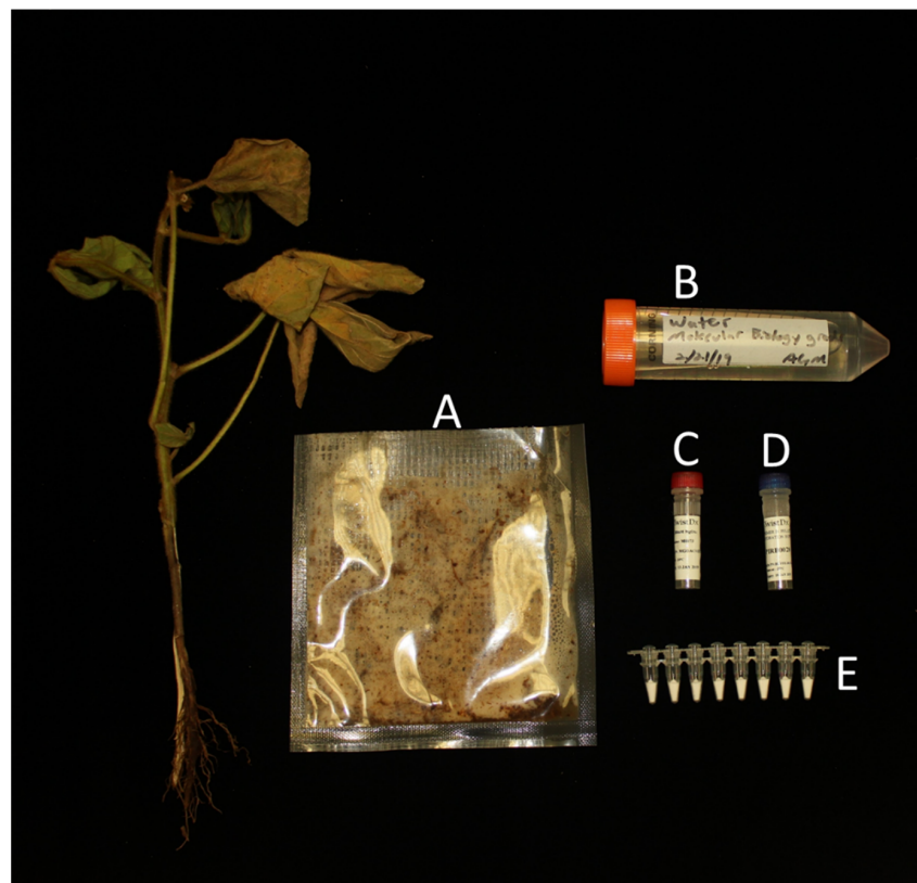
Figure 3. All necessary reagents to run the lyophilized RPA assay. (A) Crude extract produced with diseased plant sample and GEB2 buffer within an Agdia mesh bag. (B) Sterile water. (C) Magnesium acetate to initiate the reaction. (D) Rehydration buffer. (E) Preformulated lyophilized RPA reagents in pre-loaded tubes (TwistDX, Cambridge, UK).
