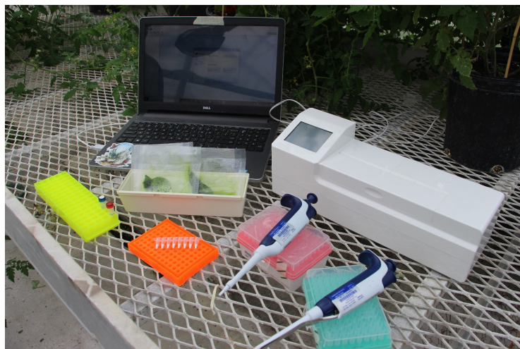
Figure 2. Visualization of the minimal space and equipment needed to perform the preformulated recombinase polymerase amplification (RPA) assay outside of the laboratory. AxxinT16-ISO used for visualization.
