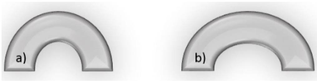
Figure 4. Crown design: (a) low and (b) high radius of curvature in the middle area of the crown.
