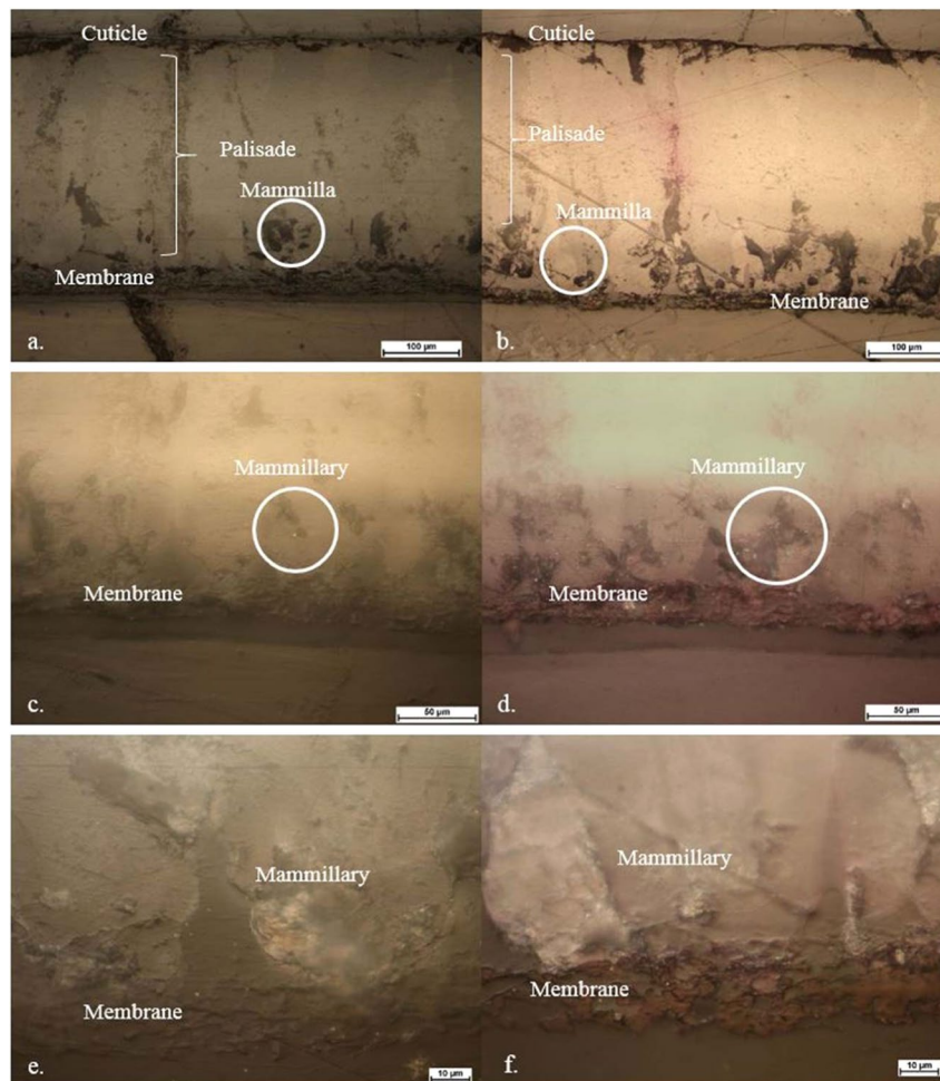
Figure 2. Polarization microscope images of thin sections from (a,c,e) the control eggshell and (b,d,f) eggshell with 2 g/L RBV-5R adsorbed.
