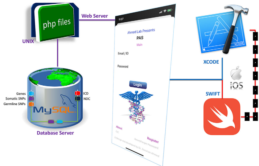
FIGURE 1 PAS components design, development, and data flow. PAS is an iOS app developed with Swift programming language, XCODE integrated development environment for MacOS, MySQL database management system, PHP scripting language, and UNIX-based web and database servers
