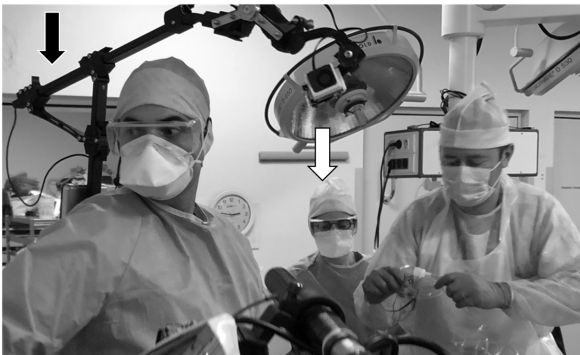
Fig. 1. Illustrates the recording hardware set up (black arrow) that are attached to the medical healthcare professional expert that performed the procedures in real-time. The medical healthcare professional is wearing a harness with an arm extending from his back permitting the recording to occur above his head during the procedures. At the tip of the arm, a case containing two cameras (white arrow) records his first-person point-of-view (FPV).
