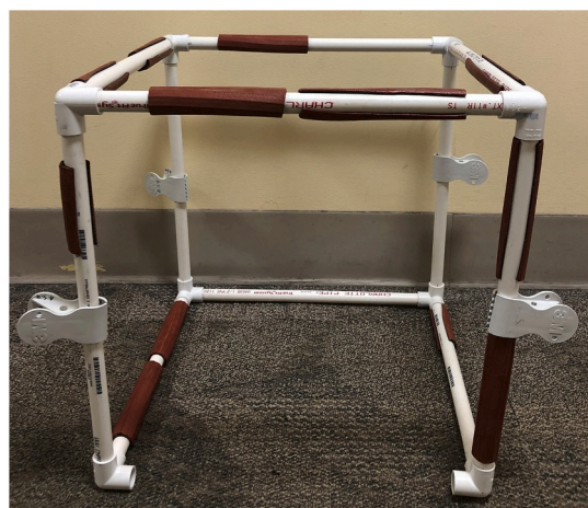
Fig. 1. Lightweight, disposable hood device with and without nylon covering.
