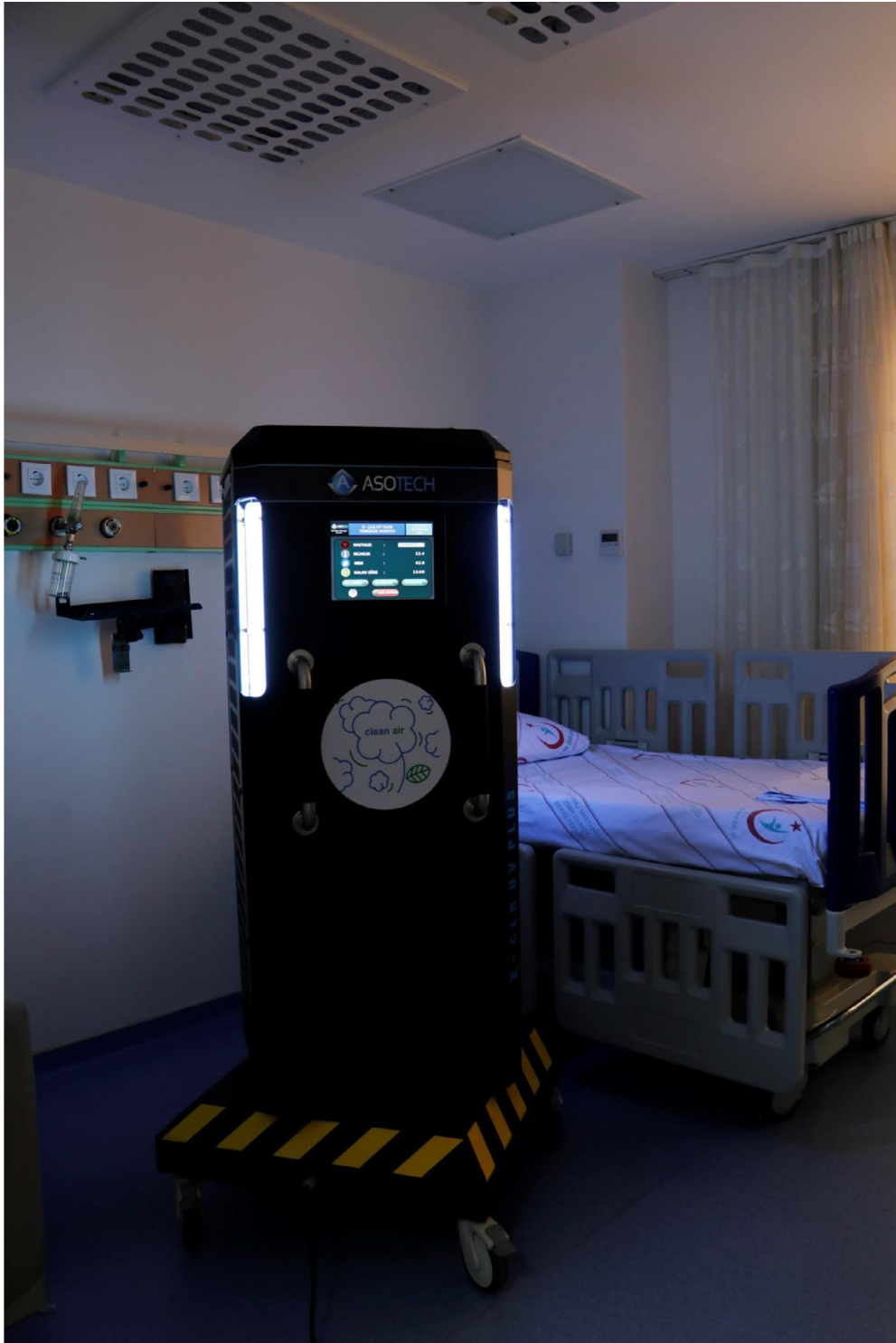
Image 2. Multifunctional UV disinfection robot with air-cleaning properties used in addition to disinfection of the physically cleaned rooms.
