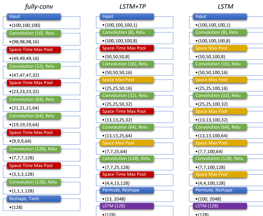
Figure 4. Architecture of the video branch f_{\text{sil}}(\cdot) for the three networks tested in this work. The other branches f_{\text{bb}}(\cdot) and g(\cdot) present the same architecture with 3D operators replaced by the 1D counterpart.
