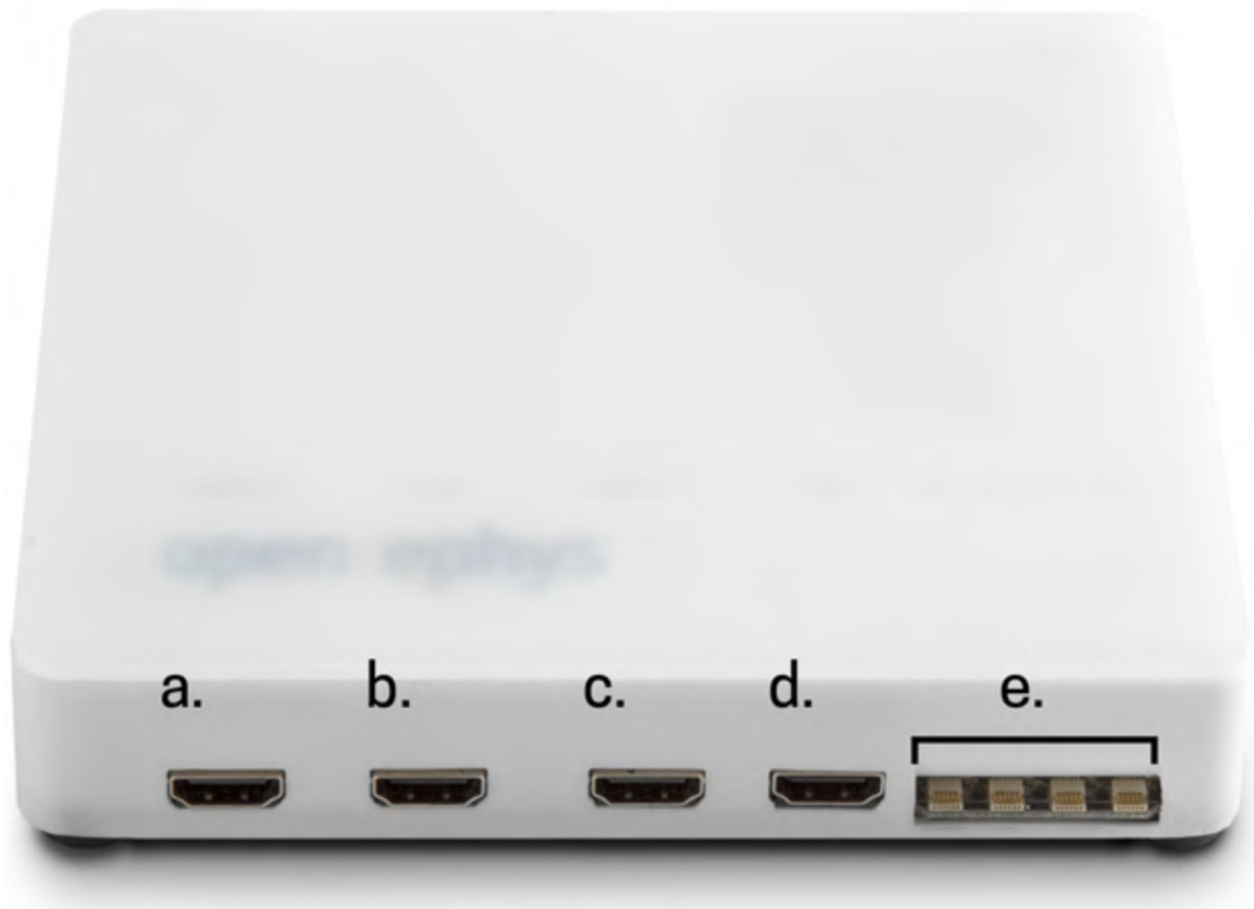
Figure 3. Input and output connections of Open Ephys Acquisition Board. a) \pm 5V analog output, b) \pm 5V analog input, c) 0/5V digital output, d) 0/5V digital input, e) SPI terminal for connecting to Intan based headstages. Photoadapted from www.open-ephys.org .
