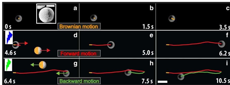
Fig. 1 Reversing the propulsion direction using different wavelengths of light. a–i Time-lapsed bright field microscopy images are showing the mode of the motion and the overlaid trajectories revealing the typical trajectories, respectively. The half-Au-coated anatase TiO 2 particles are dispersed in 12 vol% H 2 O 2 solution. Note the bright side is the TiO 2 side while the dark side is the half-gold-coated cap. In the schematic, the gold colour corresponds to the gold-coated side of the particle, whereas the light brown represents the sintered TiO 2 . Colour of lightning bolt illustrates the wavelength of light used in the experiment. a–c Brownian motion of the particle. Inset shows a scanning electron microscopy (SEM) image of the Au-coated TiO 2 Janus particle. d–f The swimmer propels in the forward direction under illumination UV light. g–i The swimming direction of the particle is reversed after a switch to green light. The arrow depicts the direction of the propulsion. The brightness and contrast of the images are adjusted using ImageJ. Scale bar is 5.0 μm. Scale bar in the inset is 2.0 μm.
