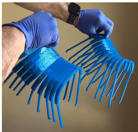
Fig 2. Left: 10 printed frames without 3D printing supports being removed from the printing bed with a spatula. Right: 20 3D printed frames; note they come together and are easily detachable. 3D, 3-dimensional.
