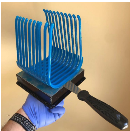
Fig 2. Left: 10 printed frames without 3D printing supports being removed from the printing bed with a spatula. Right: 20 3D printed frames; note they come together and are easily detachable. 3D, 3-dimensional.
