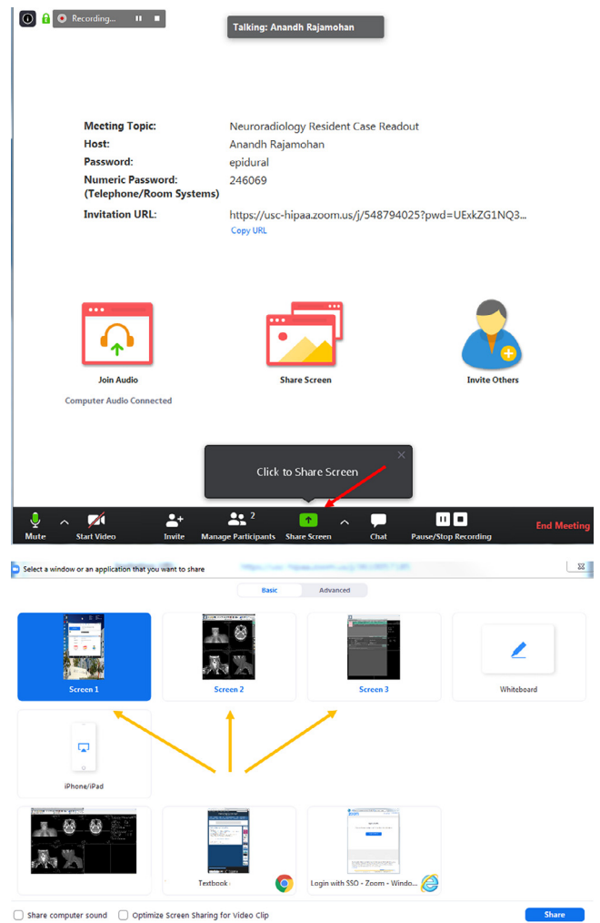
Figure 4. Screen-sharing options. (a) After the host radiologist launches the read-out session, she or he will have the option to share their PACS screen (red arrow) or any secondary screens to the remote viewers. (b) This screen-sharing function can be switched throughout the readout as needed (orange arrows). For example, the read-out session may involve a CT of the abdomen and pelvis for a patient with right lower quadrant abdominal pain with an incidental adrenal nodule. The host radiologist may want to switch the shared screen from the PACS to a webpage with an adrenal washout calculator, so all of the residents can see how the calculation is done. This screen-sharing function can also be given by the host to others who are involved in the readout remotely. For example, for the case discussing the adrenal nodule, a remote resident may bring up a good review article to show others in order to supplement knowledge on this topic. (Color version of figure is available online.)
