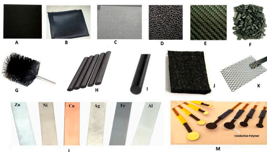
Figure 3. List of commonly used electrodes: (A) carbon paper, (B) carbon cloth, (C) carbon fibre, (D) reticulated vitrified carbon, (E) carbon mesh, (F) graphitic granular, (G) carbon brushes, (H) graphite rod, (I) polycrystalline graphite, (J) carbon felt, (K) platinum mesh, (L) different metal electrode strips, (M) conductive polymer-based strips.
