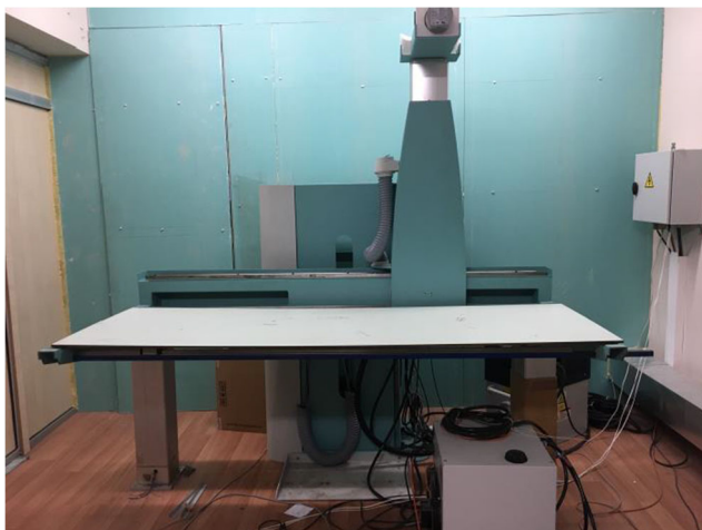
Fig. 8 Developed full-body X-ray scanner. In this device, a TDI detector, high-frequency power generator, and three servo motor drivers are required to be controlled with iBEX
