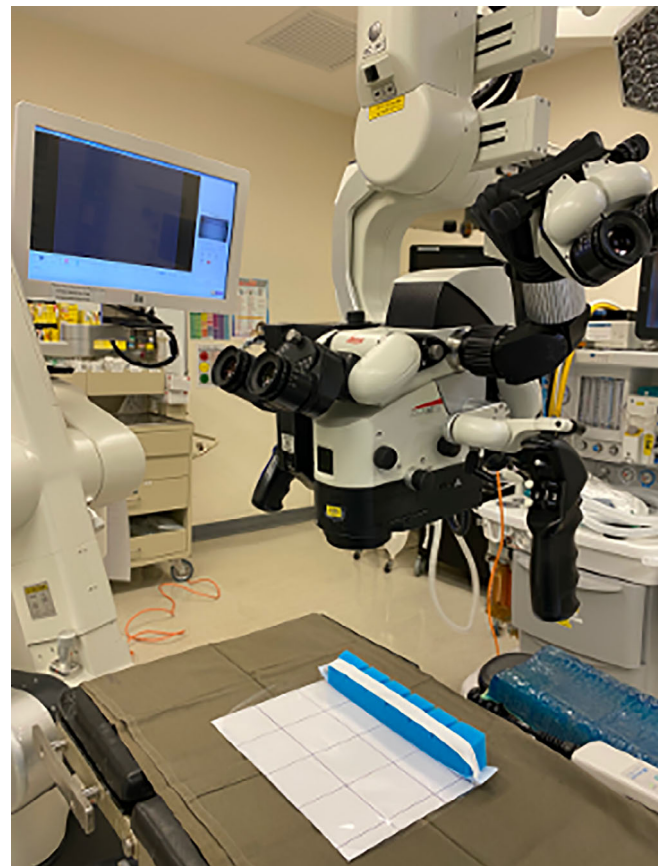
FIGURE 1 Face shield placed on white background with grid prior to droplet count with surgical microscope [Color figure can be viewed at wileyonlinelibrary.com ]
