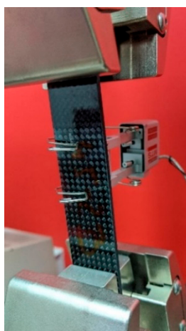
Figure 3. Photograph of experimental verification of computed mechanical properties of the composite rectangular samples.
