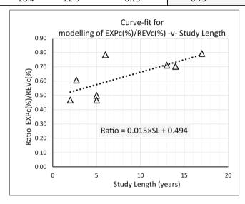
The ratio of  $EXP_c(\%)/REV_c(\%)$  was evaluated for each of the studies above. The relationship between this ratio and study period was obtained by a curve-fit as shown in the graph. The resulting linear equation was then used to model  $EXP_c(t)/REV_c(t)$  (fitted) at the respective study lengths. These fitted values were then used in the equation:  $SUR_c(t) = EXP_c(t) \left[ \left\{ EXP_c(t)/REV_c(t) \right\}^{-1} - 1 \right]$  (see text), to provide a modelled estimate for  $SUR_c(t)$
