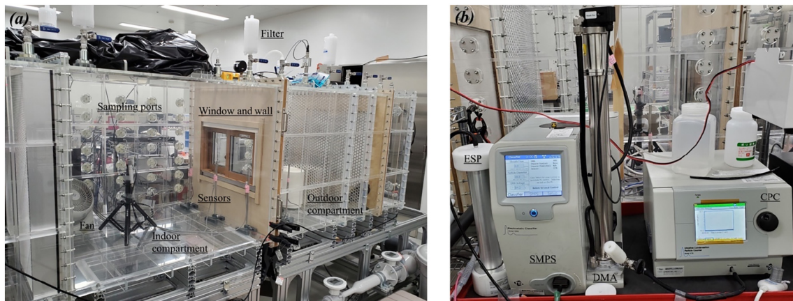
Fig. 2. Experimental photos. (a) The test chamber in simulation system (delivery pump and exhaust pump are not mentioned) and (b) CPC and SMPS with DMA in measurement system.
