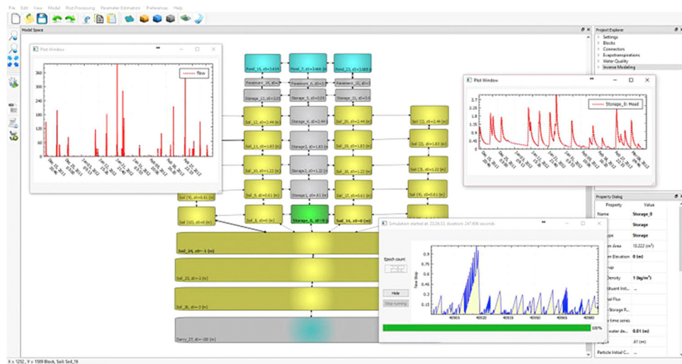
Fig. 2. A snapshot of the GUI version of the GIFMod with the model representation for the permeable pavement example.
