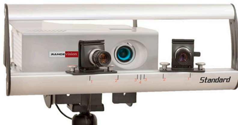
Figure 2. Three-dimensional digitizing instrument—Rangevision Professional Standard.
