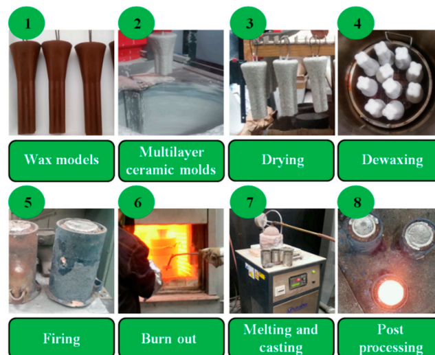
Figure 2. All stages of shell molds and castings preparation.
