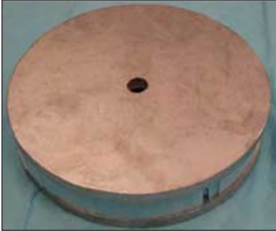
Figure 1. Photographs of specially designed cerrobend shield (22 cm diameter and 1.2 cm thickness) used to encase the body of the mice, exposing only 1 cm diameter of the lower abdomen.
