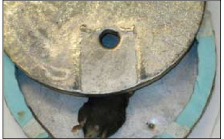
Figure 1. Photographs of specially designed cerrobend shield (22 cm diameter and 1.2 cm thickness) used to encase the body of the mice, exposing only 1 cm diameter of the lower abdomen.
