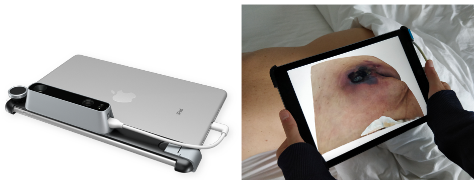
Figure 2. (Left) The Structure Sensor mounted on an iPad. (Right) Scanning of a pressure injury using the Structure Sensor.
