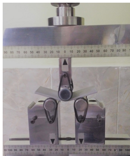
Figure 3. Three-point bending method used for mechanical properties testing.
